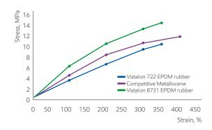
In a typical 3728 type of medium-voltage insulation formulation, Vistalon 722 EPDM rubber affords excellent flexibility in an AEIC cable construction compared with TRXLPE. Furthermore, the ethylene-propylene elastomer is much less sensitive to a decrease in temperature than TRXLPE.
